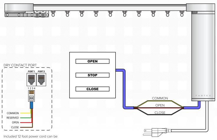
configured on-site to run off the bottom, side, or top of the motor. Low voltage line attaches to RJ-9 on the bottom of the motor, Port 1. Available with wall or
