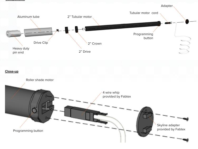
**Requires** - Standard 120VAC power supply provided & installed by EC/GC (all connections), must be hardwired. **Controls Available** - Levitron #5657 Rocker Switch (Recessed) to be provided & installed by EC/GC (or equal). **Tube Size** - Compatible with 2" Diameter Tube (Standard Crown & Drive). also compatible with 2-1/2" Diameter Tube (Requires larger Crown & Drive).
